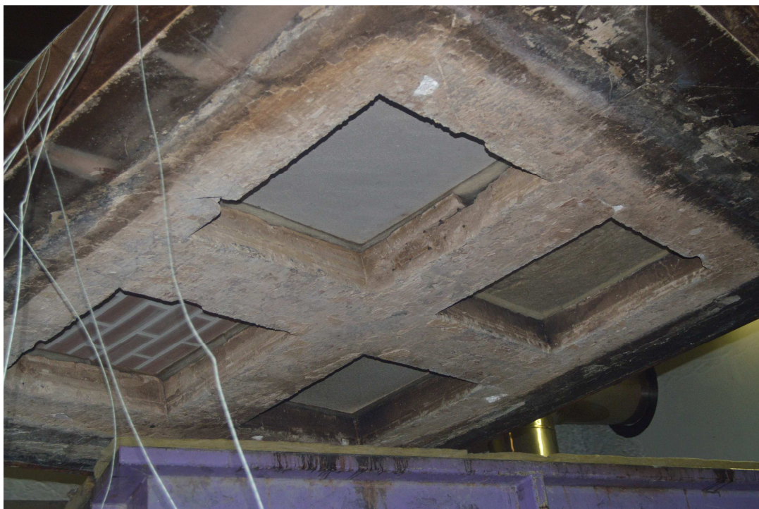
Photo No. 2 Test specimens no A1, A2, A3 and A4 seen after the test (test 1)
